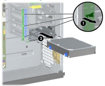
Figure 5-22 Removing a Hard Drive
